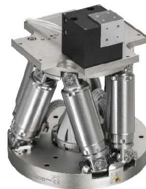
Figure 1. F-712.HU1 Fast Multi-Channel Alignment Micro-Robot. This is an assembly of a fast, high-resolution closed-loop Nanocube® piezo nanopositioner and a long-travel, 6-DOF hexapod driven by brushless DC servo-motors
